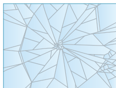
Toughened Glass Thermally Toughened glass
