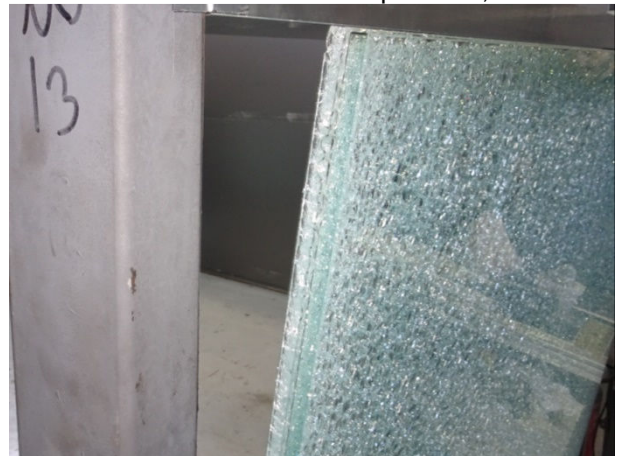
Picture 10 Fracture of the outer glass sheet at +4400 Pa
