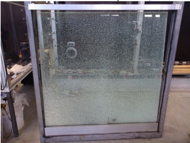
Picture 9 Fracture of the outer glass sheet at +4400 Pa
